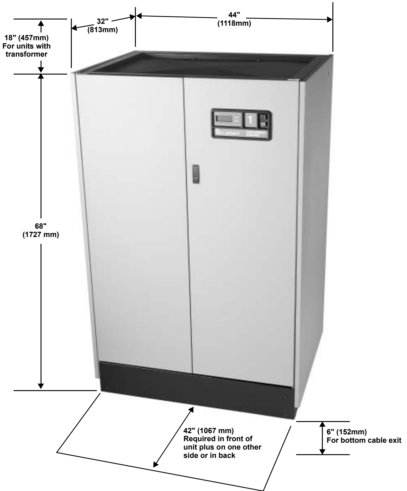
Figure 9 Dimensions, clearances, 3 panelboards
